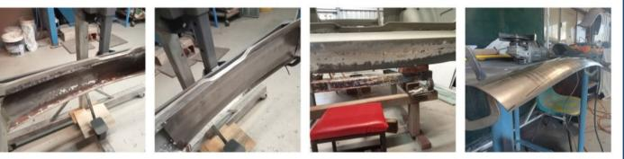
The passenger side rear quarter panel also came in for attention and repair. The completion of this work needed about 2 inches of rusted panel to be removed and replaced. A new section was shaped and carefully welded into place, then ground back smooth and primed to
