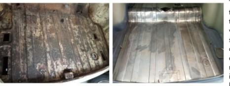
The first series of photos show the before and after picture of the boot floor. Perhaps not so visible in the first photo but this shows the boot floor with a hundred or so rust holes. The second photo shows the nice shiny new floor which Jim fabricated, including the raised ribs on the bead roller.
